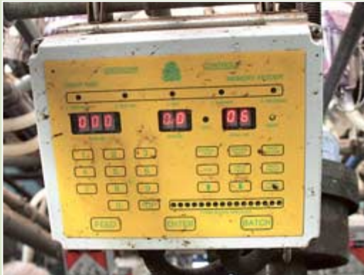
Flow meter in situ. Each unit costs about £630 installed with auto cluster removal and control box. System can be 'grown' by linking it to an office computer, which records the entire history of the cow in terms of yield, calving, milk quality etc.
