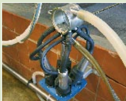
The cluster. Note the receiver that allows the volume of milk to exit via the milk pipe. Too low a capacity, and the milk from one quarter can 'jet' up another teat cup and make contact with another quarter – risk of cross contamination etc. See also the twin pulsator lines; these should be the same length.
