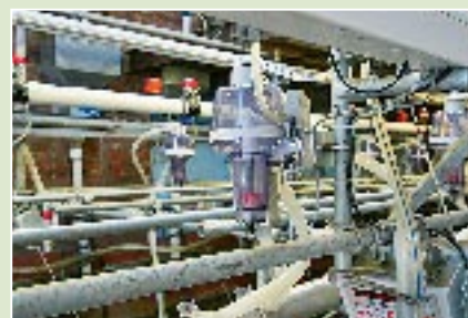
Milk recording jars have no place in modern parlours. Jars should be replaced with electronic systems that measure milk flow and do not affect vacuum pressure.
